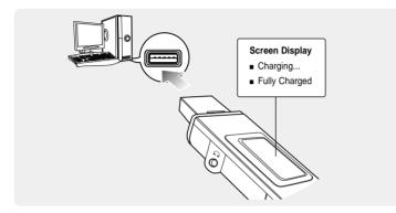
Remove the USB Cover and then connect the USB Connection Plug to the USB port  $({\mathfrak q}_{7})$  on your PC.
